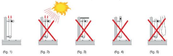
It is of fundamental importance that thermostatic kits do not are then installed under barriers, such as shelves, curtains, movable or mounted vertically.
